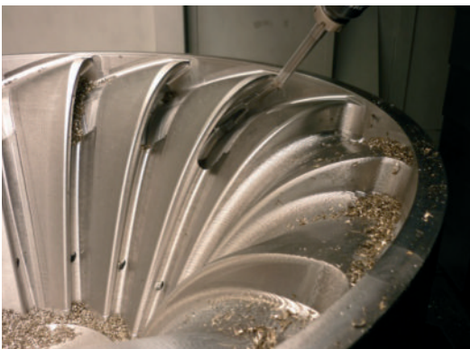
From top left, counterclockwise: Partially machined solid steel block before milling; Francis turbine partway through milling process; 5-axis CNC mill in the finishing stages of manufacturing. All photos from the Benesov, Czech Republic facility.
